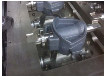
Casting in mold with core pin
